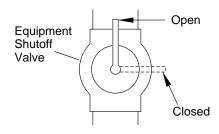
Figure 22 - Equipment Shutoff Valve
